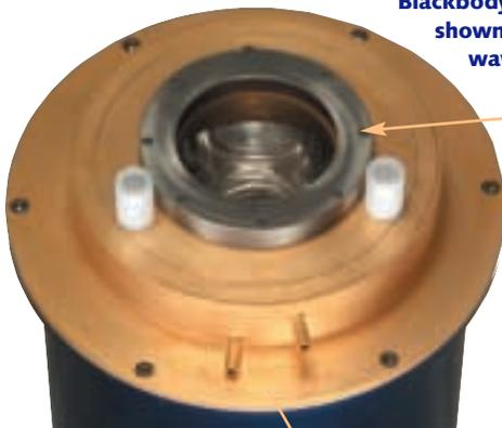
**Blackbody cavity shown without waveguide horn**
